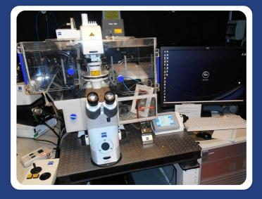
Traditional fluorescent microscopy relies on a single emission filter to select an output range. Spectral detection allows for the acquisition of data across a range of wavelengths, accumulating more of the emitted light.
