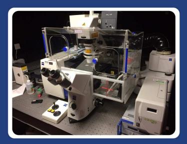
Unlike traditional fluorescence microscopy, **multiphoton** (MP) microscopy excites samples with a lower-energy laser for reduced scattering, less bleaching and greater sample penetration.
